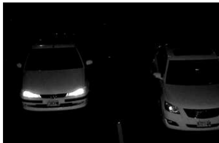
Clear Image Captured with IR Illuminators and Headlight Filter
